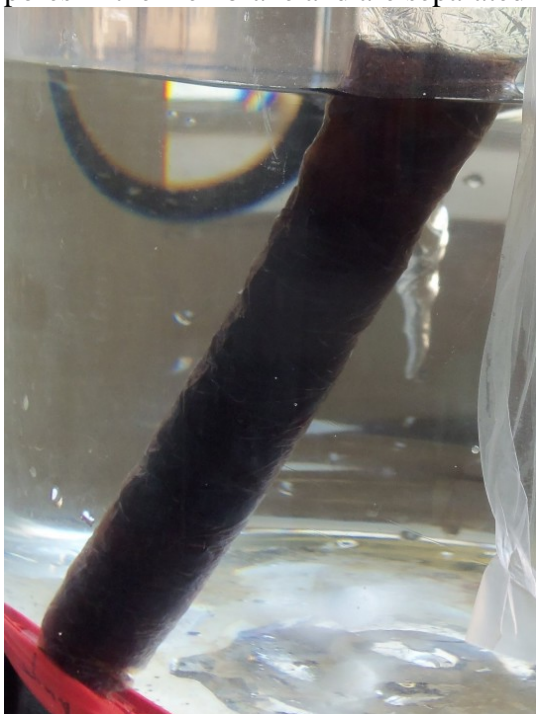
Figure 4.16 – A brown suspension of carbon nanoparticles in a tubular dialysis membrane. The nanoparticles cannot pass through the pores of the membrane, but water molecules can pass.
