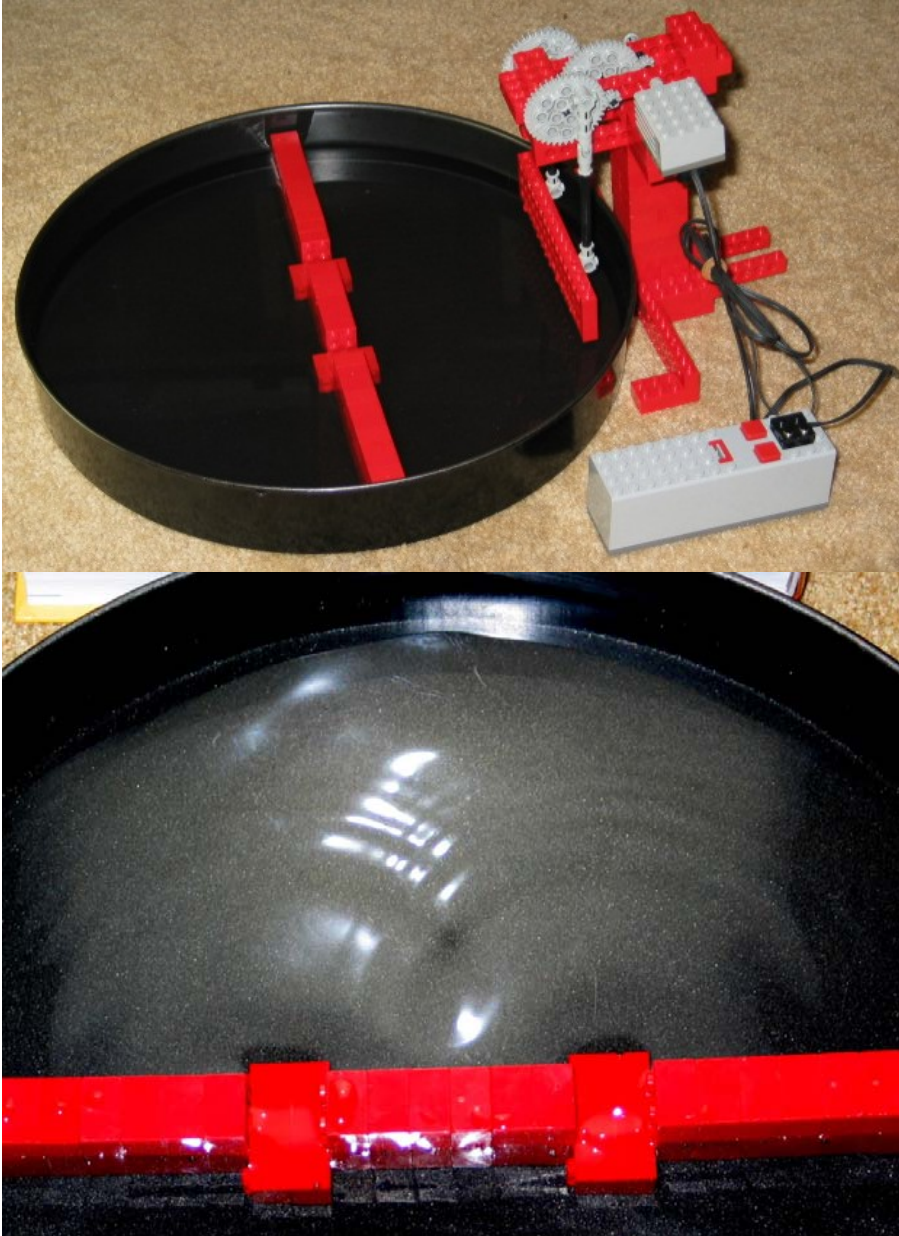
Figure 2.21 – (top) A wave tank made using LEGO® bricks and a flat pan filled with water. A long, straight wave can be produced by oscillating a flat wall of LEGO® bricks. The wall can be oscillated up and down by using a LEGO® machine or by hand. (bottom) Interference between sets of circular waves scattered from two gaps in the 2x4 LEGO® brick barrier. The water level is lower than the bricks oriented vertically but higher than the bricks in the gaps that are oriented horizontally.
