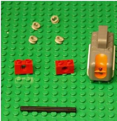
Sensor & Mount Parts: 2 1x2 Technic bricks, 1 cross axle #6, 4 1/2 bush pieces 1 light sensor
