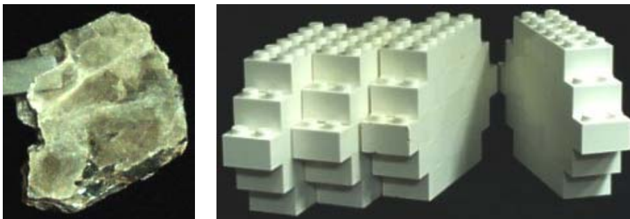
Figure 3.9 - (left) A mica mineral. (right) A LEGO® model of the mica structure made from brick walls of 19 2x2 bricks. Note that the walls can peel away from each other to model the sheet-like structure of mica.
