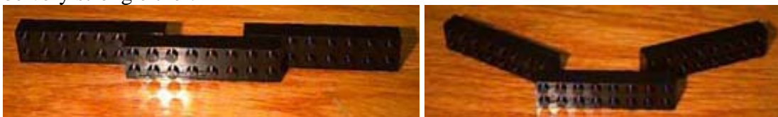
Figure 3.13 – (left) Beam of Material B made from three 2x8 bricks. (right) Distorted beam of Material B.
