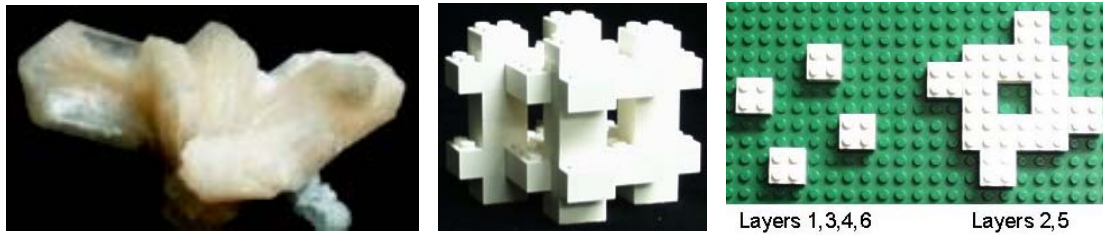
Figure 3.10 - (left) A zeolite mineral. (middle) A LEGO® model made from 40 2x2 bricks of a three-dimensional structure that is reminiscent of a zeolite, which features three channels, all perpendicular to each other. (right) The layers used to produce the LEGO® structure.
