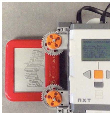
Figure 8. The NXT Controlling an Etch-a-Sketch
